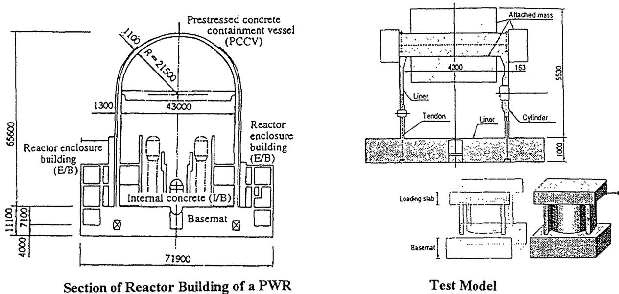
Fig.5 Outline of Actual PCCV and Scaled Test Model.
