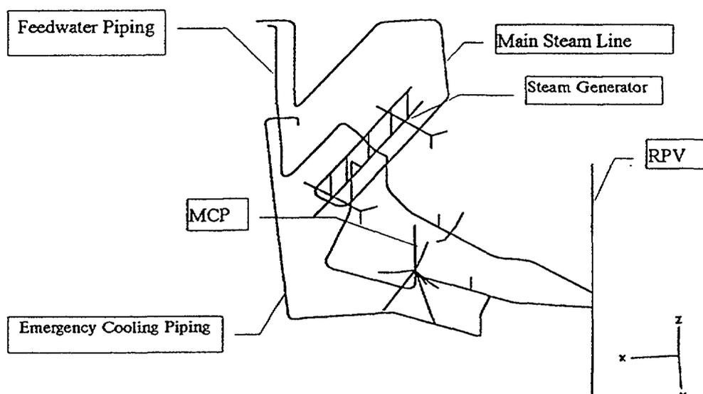
Figure 2 Analytical Model of the first PCLS
