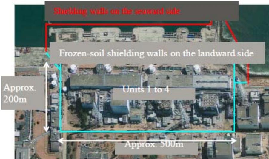
Plan of Shielding Walls around Buildings
