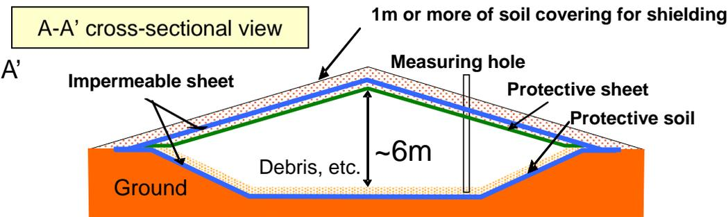
Shielding with soil (debris)
