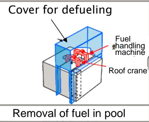
Feasibility of retrofit cover for debris removal (seismically safe construction)
